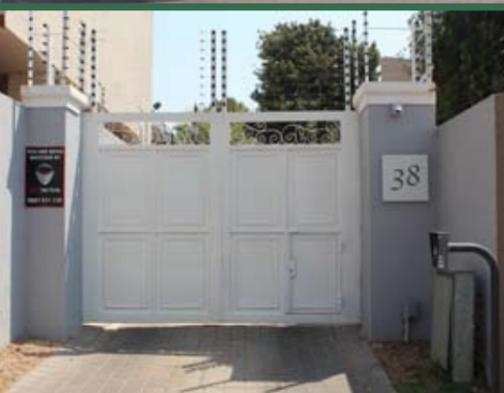
Above: Automated double swing gates integrated with a CCTV surveillance system and Centurion Polo GSM intercom, and electric fencing at a private residence.
